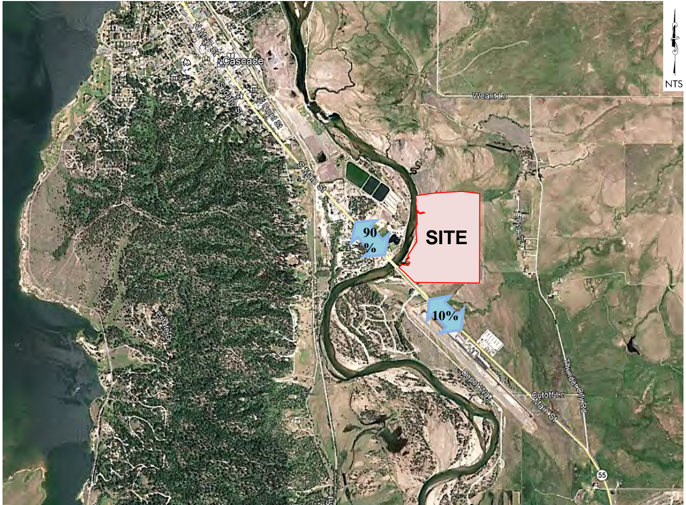
Figure 4.1 – Site Traffic Primary Trip Distribution Patterns
